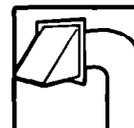
Is exhaust duct or outside exhaust hood clogged with lint?
